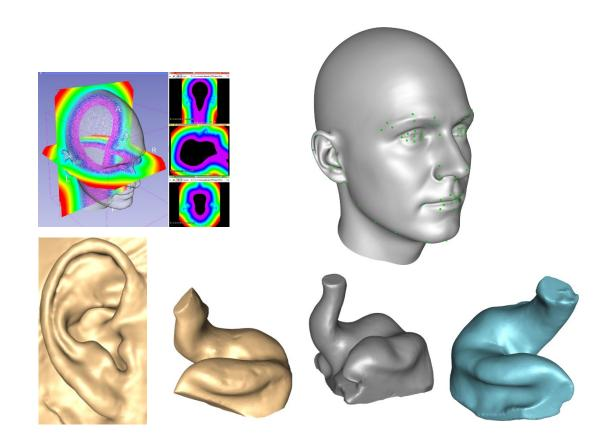
• Statistical shape models for hearing aid design and acoustical simulations
