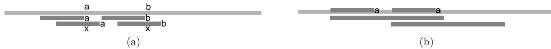
Fig. 3. The new string-matching algorithm using slubs: (a) sparsify to one candidate in each |z| + 1 block: after verifying the size 2 deterministic sample \{a, b\} , any surviving occurrence candidate that has another close-by candidate on its left, can be eliminated. (b) sparsify to one candidate in each period length \pi(x) block: after verifying the deterministic sample za , any surviving occurrence candidate that has another close-by candidate on its right, can be eliminated.
