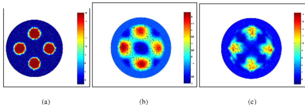
Results of reconstruction of simulated data (a): True model, (b): Image reconstruction using Tikhonov regularisation and (c): TV regularisation with noise free data
