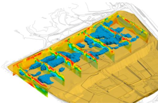
A three dimensional ERT survey of a commercial landfill site to map the volumetric distribution of leachate (opaque blue). Leachate is abstracted and re-circulated to further enhance the production of landfill gas, and subsequently the generation of electricity. This image was provided by the Geophysical Tomography Team, BGS, and is reproduced with the permission of the British Geological Survey ©NERC. All rights Reserved.
