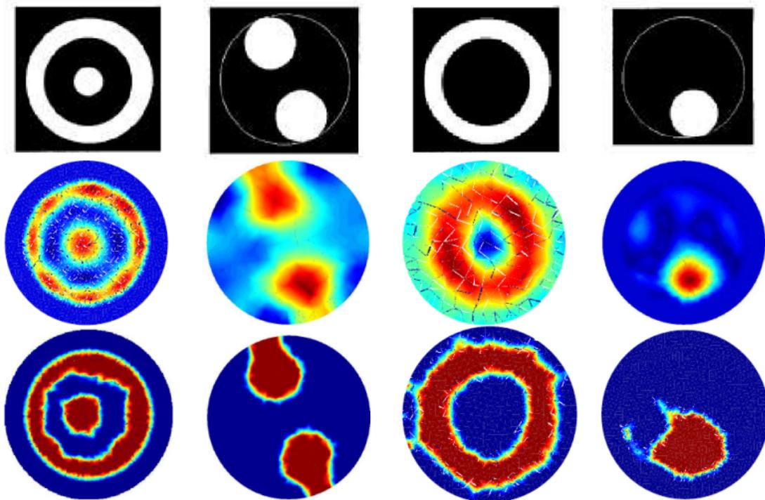
Level set reconstruction for experimental ECT data. The region of interest is the interior of the pipe. In the images 2 and 4 only the inside of the pipe shown, whereas in the images 1 and 2 the exterior part is also shown. The top row shows the real object, the center row the pixel based reconstructions, and the bottom row the shape based reconstructions.
