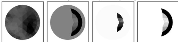
Barrier example: (a) Gauss-Newton reconstruction and then (b) posterior mean resistivity, (c) posterior standard deviation, and (d) posterior "probability of being inclusion".
