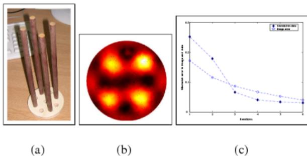
Reconstruction of 4 plastic rods shown in (a) from experimental data shown in (b) and the norm of the mismatch error between measured and simulated normalised capacitance shown in (c)
