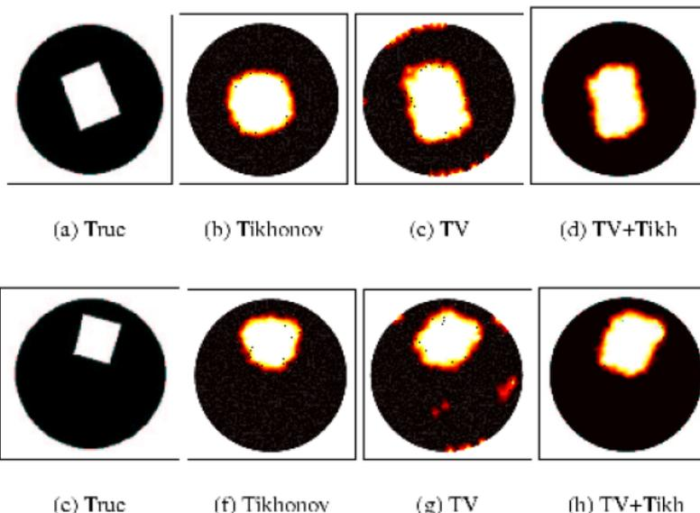
Reconstruction of wood with square cross section (permittivity 2), using TV and Tikhonov regularisation, We would like to thank M. Byars of Process Tomography Ltd. Wilmslow Manchester UK, for this ECT experimental data.
