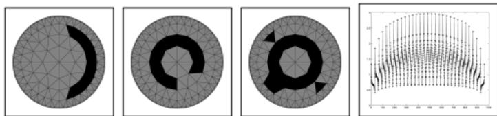
True inclusions: (a) *Barrier*, (b) *C-Shape* and (c) *Ring*, and (d) measurements from Barrier for a 32 electrode system.
