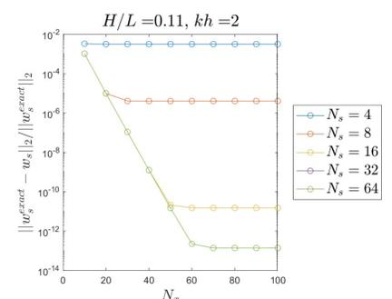
Figure 3: The convergence of  $w_s$  as a function of  $N_x$  for different values of  $N_s$ .
