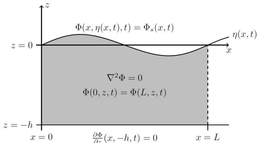
Figure 1: An illustration of the physical system for a flat seabed,  $h(x) = h$ .
