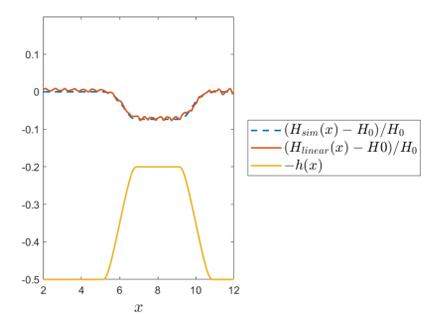
Figure 5: The simulated and expected relative wave height  $(H(x) - H_0)/H_0$  for linear waves propagating over a barrier.
