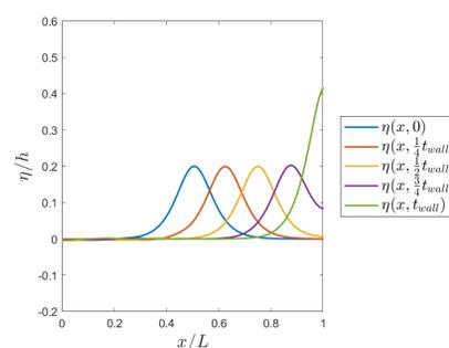
Figure 4: A solitary wave with initial amplitude  $0.2h$  running into a wall at different instances of time.
