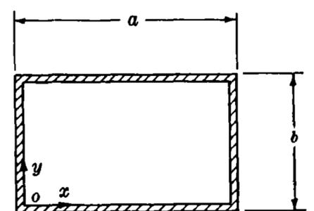
FIG. 2-1.—Rectangular waveguide cross section.
