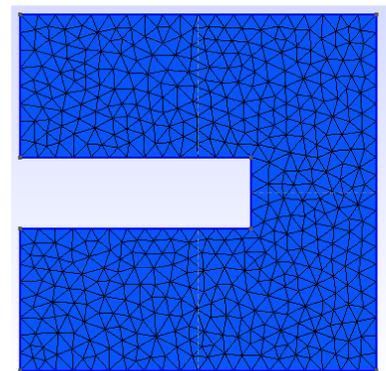
Figure 3: Waveguide cross section defined and meshed in Gmsh. The dimensions from the bottom left to top right corner are 20 by 20 mm.
