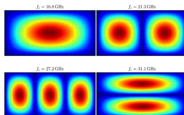
Figure 2: FEM solution for the four first modes in rectangular waveguide of dimensions  $a = 20$  mm and  $b = 10$  mm (see Figure 5).
