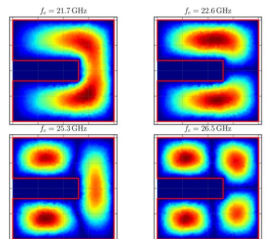
Figure 4: First four eigenmodes for the geometry in Figure 3 (Note that the used mesh was finer).
