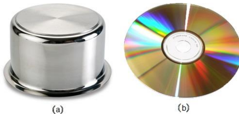
Figure 10: (a) A real life brushed metal object showing long anisotropic reflections across the entire surface. (b) A compact disk showing light diffraction effect on an anisotropic surface.
