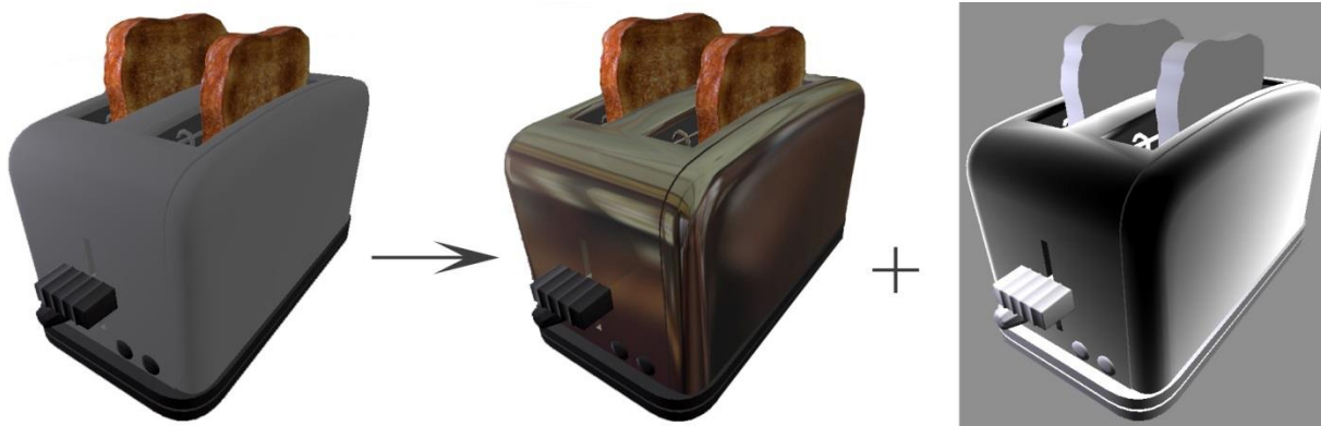
Figure 31: The plain diffuse component applied to a 3D model of a toaster on the far left. A cube map reflection applied to the model in the middle render and just the Fresnel term contribution on the far right.
