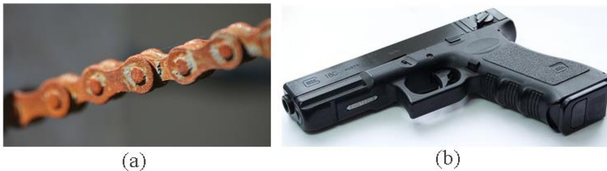
Figure 18: (a) An example of the most common type of rust – red rust. (b) Black oxide also known as black rust. Often used as a protective coating against red rust.
