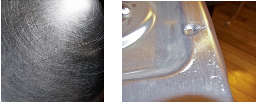
Figure 12: Real world metal materials showing isolated scratches on their surfaces. On the left there is an interior bottom of a steel cooking pot. Scratches got there from scrubbing and cleaning the cooking pot with a metal brush sponge. On the right side there is a picture of a kitchen sink.
