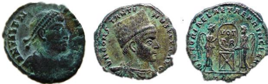
Figure 25: Bronze coins with engraving on the surface demonstrating the formation of metallic patina in the low point areas (cracks, creases, and cavities).
