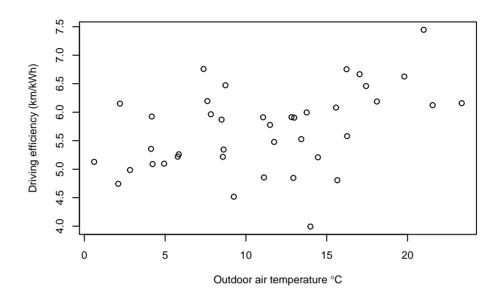
A simple linear regression model with the driving efficiency as model output, and outdoor air temperature as model input, was fitted. The results were:
