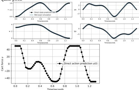
The curves show the direct methods predicted trajectory (i.e. what the optimizer think will happen) as well as the true trajectory as obtained by RK4 integration (there are two curves, they just agree!). Other plots, not shown here, will show the defects, i.e. how much the equality constraints in the collocation are violated. The defects should be small, otherwise the optimization has failed.
