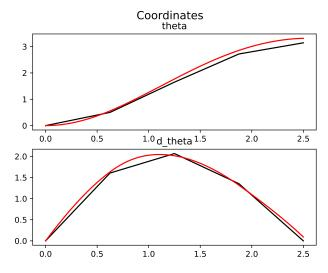
It shows how well the solution of the path  $\boldsymbol{x}(t)$  found by the direct method you just implemented matches the solution obtained by taking the control signal you found from the solver,  $\boldsymbol{u}(t)$ , and simulating it in the real system using the RK4 scheme. We see the solution actually works: it brings the pendulum to the right place. However, the mesh is so coarse the quality of the solution is not great. Try to increase N=20 to see how that solves the problem.
