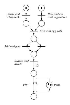
Remarks: Whether to add maizena or not is represented by a choice with a void branch. The the crossed arc with a 10 represents 10 arrows corresponding to the division into portions. According to the way we define simultaneous firings of a transition with itself, the last part allows for frying two pancakes at a time.
