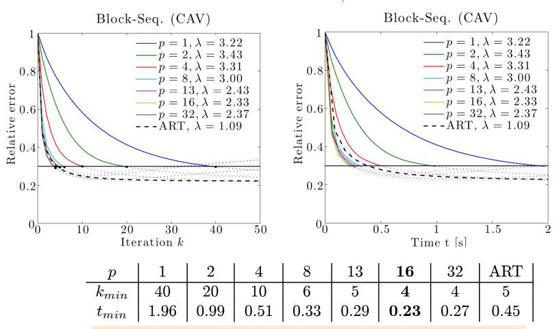
The advantage of "block sequential" over standard ART is due to the improved use of the multicore architecture.
