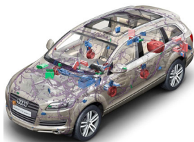
Figure: ECUs interconnected inside a vehicle 2
