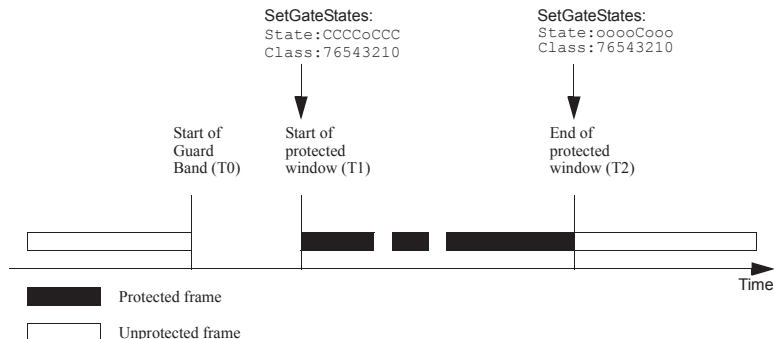
Figure 2.4: Protected window using gates [12]
