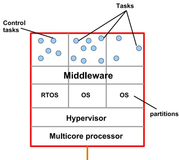
FIGURE 2. Fog node architecture. The software stack is running on a multicore, and has, from bottom to top, a hypervisor, partitions running OSes, middleware and tasks.
