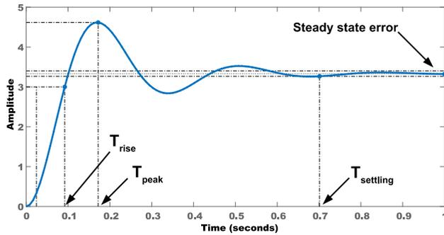
FIGURE 7. Step response of a sample control loop.
