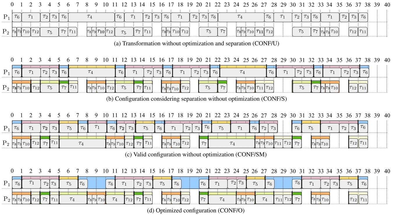
**FIGURE 8.** Four different configuration for the applications in Table 2; The black lines show the overheads of the partitions: CONF/U has no temporal separation; CONF/S has several deadline misses; CONF/SM is feasible and the cost function value is 0.13522; CONF/O is the final solution which shows 77% improvement.
