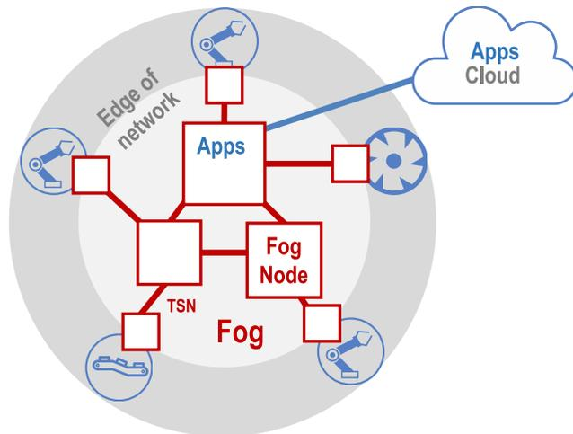
**FIGURE 1.** Fog Computing platform. Boxes represent fog nodes, connected with each other and to the Cloud; the thick lines are the network. Applications (Apps) run in the fog and Cloud.
