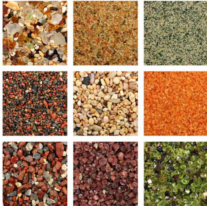
Figure 2.1: Close up of different types of sand [6]. From top row to bottom row, left to right; (1) glass sand (Kauai, Hawaii), (2) dune sand (Gobi Desert, Mongolia), (3) quartz sand with green glauconite (Estonia), (4) volcanic sand with reddish weathered basalt (Maui, Hawaii), (5) biogenic coral sand (Molokai, Hawaii), (6) coral pink sand dunes (Utah), (7) volcanic glass sand (California), (8) garnet sand (Emerald Creek, Idaho), (9) olivine sand (Papakolea, Hawaii).
