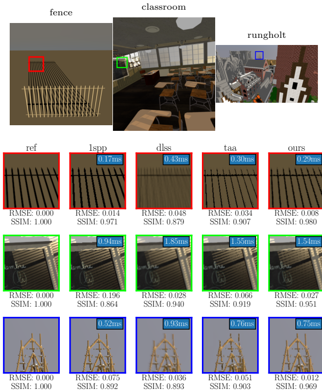
Figure 4: The three test scenes used for testing TAA performance. First scene is a static view of a fence with its moving shadow. Second scene is a sequence of VR poses in a classroom scene. Third scene is a smooth camera movement through a Minecraft map. The closeups show quality comparisons of our adjusted temporal antialiasing to conventional TAA with neighborhood clamping as well as DLSS. Our method specifically improves moving shadows and fine geometry that is far away.
