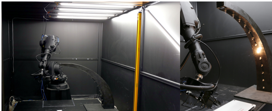
Fig. 1. Left: robotic arm holding a camera in a lightproof enclosure. Right: light arch and camera system measuring the BRDF of an aluminum laptop.
