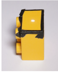
Fig. 8. Photo of a yellow toy brick made from ABS polymer. A point light source is positioned directly opposite the camera. Two diffuse light sources, positioned above and below the camera, illuminate the brick from the front. The specular highlight due to the point light is clearly visible on the top surface. The image is slightly blurred due to use of a wide aperture. Black tape was added to remove glares from the edges.
