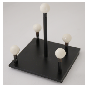
Fig. 7. 3D artifact used for camera pose estimation.
