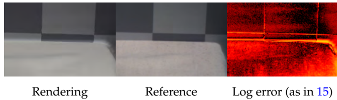
Fig. 20. Material transitions: error lines along checker edges and along the boundary between tablecloth and backdrop.
