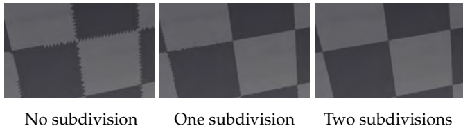
Fig. 7. Subdividing the mesh dissolves unwanted boundary sawtooth artifacts that originate from the BRDF labeling.
