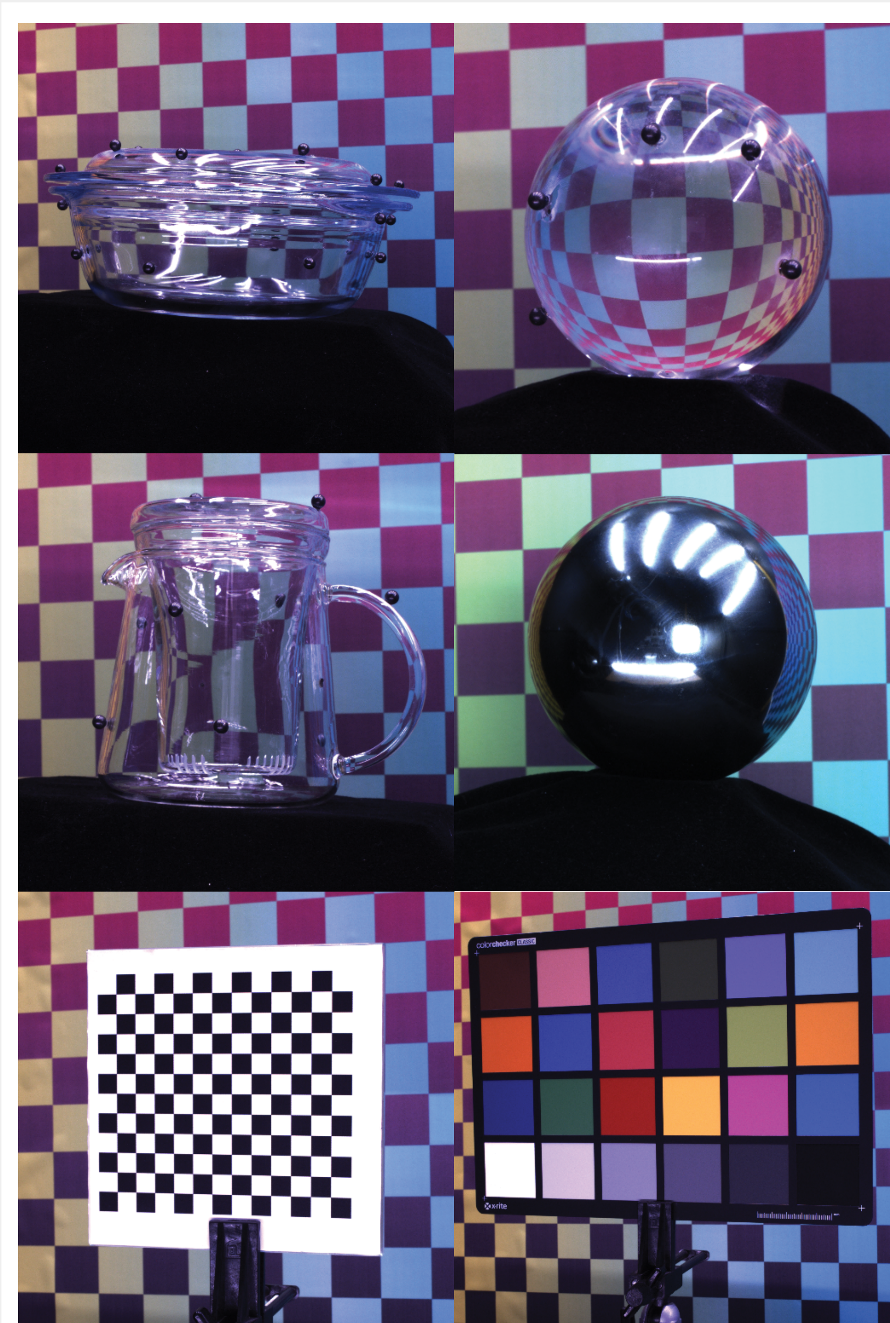
Figure 1. Preliminary images from our data set. Glassobjects: bowl, sphere, teapot) with markers placed on. Hereafter, three calibration and rendering tools part of the pipeline: chrome sphere (environment light evaluation), a black and white checkerboard (coordinate estimation), and an X-Rite ColorChecker®.
