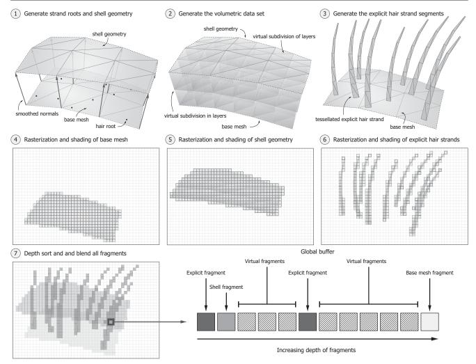
**Fig. 3** Overview of our shader pipeline. In steps 1–3, we generate explicit hair strand and shell geometry. In steps 4–6, the generated geometry is rasterized and shaded (see also Fig. 4 and Section 3.1-3.2). In step 7, the shaded fragments are depth sorted and blended in accordance with our blending algorithm (see also Fig. 5 and Section 3.3).
