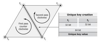
Fig. 7 Creation of unique keys for edges in order to build a neighbor data structure.
