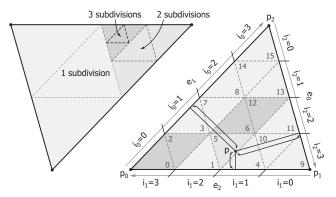
Fig. 6 Our indexing scheme for a volumetric layer.
