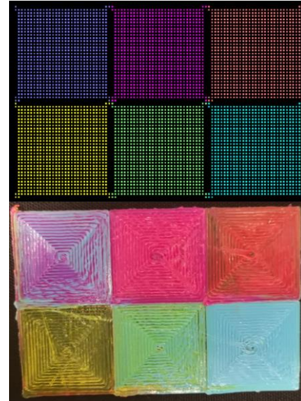
FIGURE 6: G-code points of six squares in the visualization tool (top). Six 3D printed squares without purge tower (bottom).
