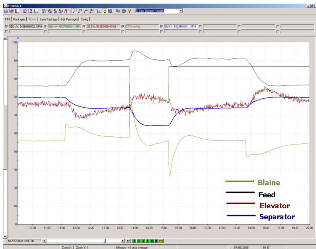
Figure 6.1: Performance of MPC with grindability factor of 36 without measurement noise(Sepax Power Changed from 330-360 Kw - Green line).
