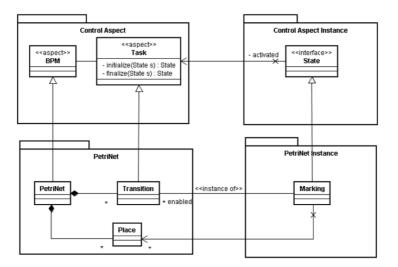
Figure 2.8: Meta-model for a Petri net implementation of the Control Aspect (image: [2]).
