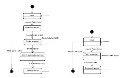
Figure 2.10: Automatas for case in the core (left) and for case in the control aspect (image: [2]).
