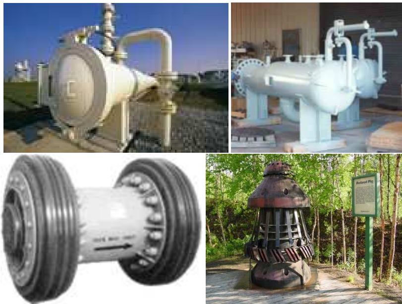
Fig. C.9. To be treated in a later version of this report: Pig Launcher, Receiver and New and Old Pigs
