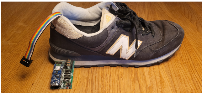
Figure 2: Shoe wearable designed for acquiring the plantar pressure and the accelerometer sensor readings for biometric purposes [41].
