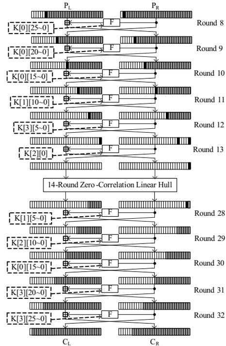
**Fig. 6.** Key recovery for 25 rounds of XTEA. For the estimation of correlation, grey and black bits need to be computed and white bits are irrelevant. Uses the zero correlation approximation of Figure 3.
