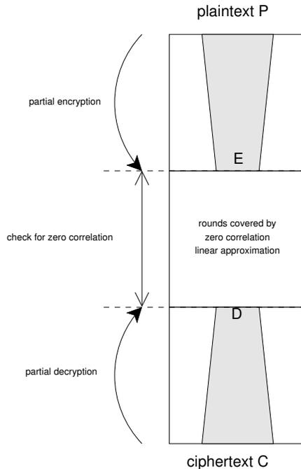
**Fig. 1.** High-level view of key recovery in zero correlation linear cryptanalysis
