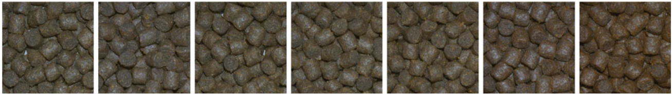
Fig. 10 RGB representation of cropped SuperK images of the pellets with seven different levels of synthetic astaxanthin coating concentration. From left to right: 0, 3.125, 6.25, 12.5, 25, 50, 100 ppm
