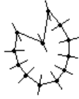
Figure 1.5: A shape model with overlaid 1D pixel profiles normal to the boundary.
