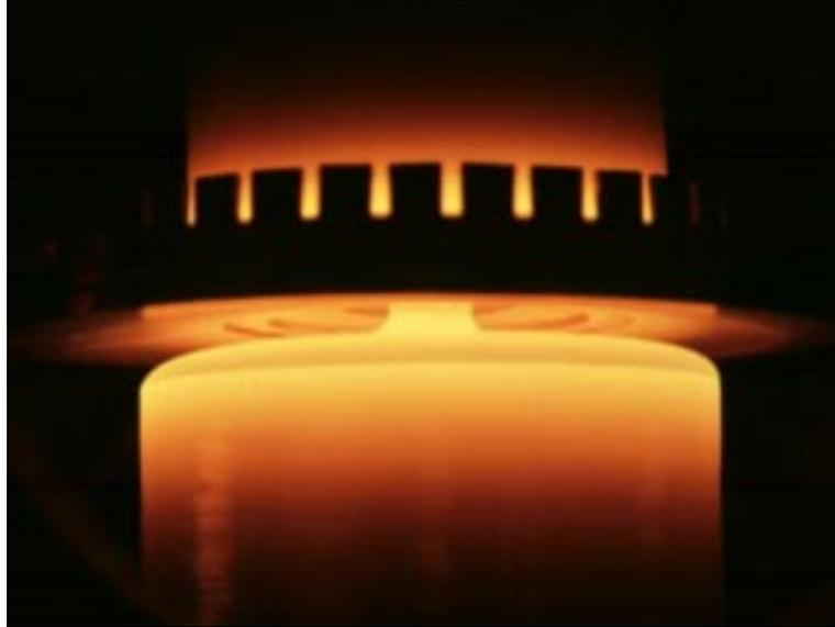
Figure 1.1. *Photograph of the IKZ 4" float zone process with courtesy of IKZ.*
