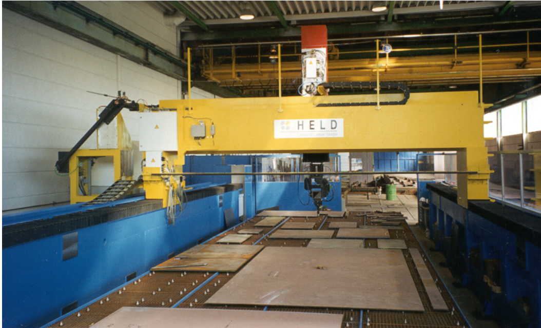
Figure 12.1: The laser cutting and welding installation. The table measures approximately 4500\text{ mm} \times 18000\text{ mm} .
