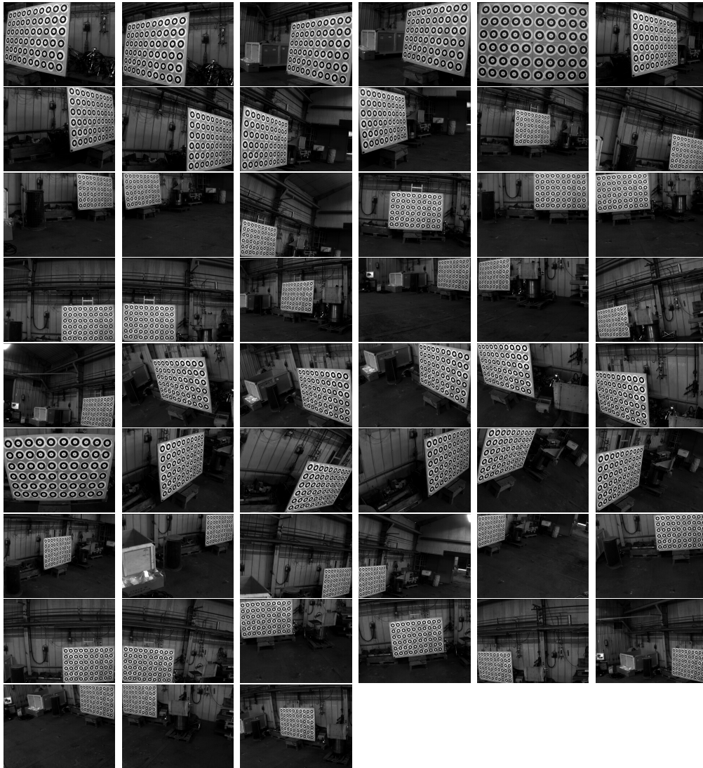
Figure 6.1: Calibration Images. The plate contains 60 coplanar calibration points and measures approximately 1400\text{ mm} \times 2000\text{ mm} .
