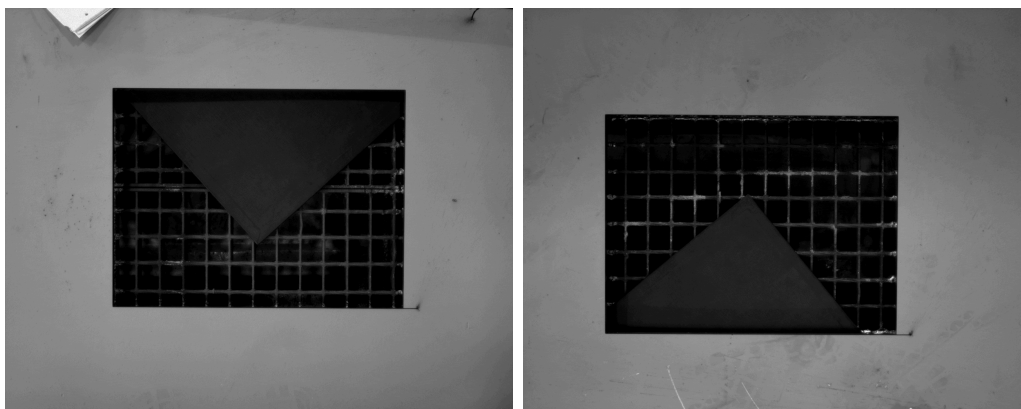
Figure 12.7: The two rectified images that are used for the external camera calibration on the laser cutting installation.
