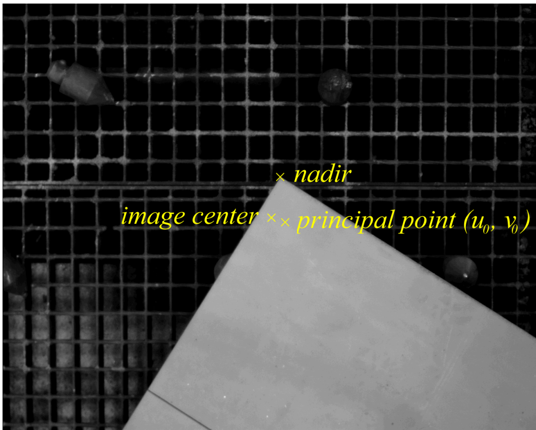
Figure 12.8: Image center, principal point, and nadir in an image from the laser station.
