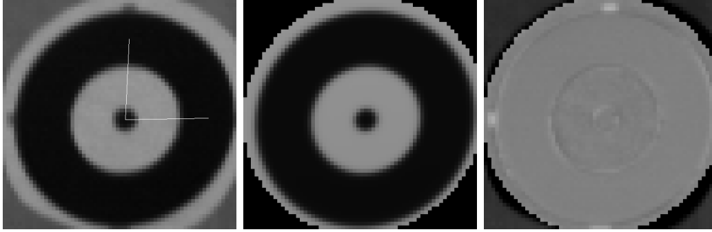
Figure 7.4: Example of circle detection. Left: original image with horizontal x -axis and vertical y -axis. Middle: the fitted model. Right: the difference between the model and the image, i.e. the fitting residual. The artifacts on the outer radius of the mark are the line segments that were used to position the mark on the graph paper.
