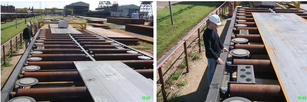
Figure 11.2: The check-in station on the quay. The large and small reference marks have a diameter of 330\text{ mm} and 110\text{ mm} , respectively.
