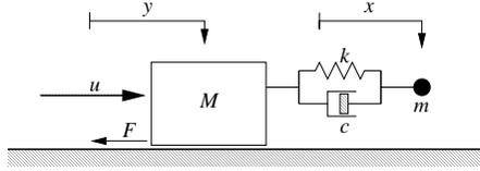
Figure 3.1: A position regulator with parasitic dynamics
