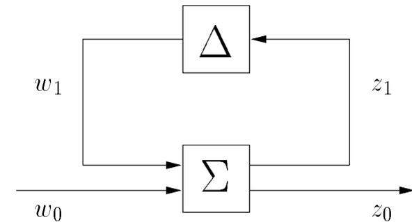
Figure 6.1: Setup for robust performance analysis.
