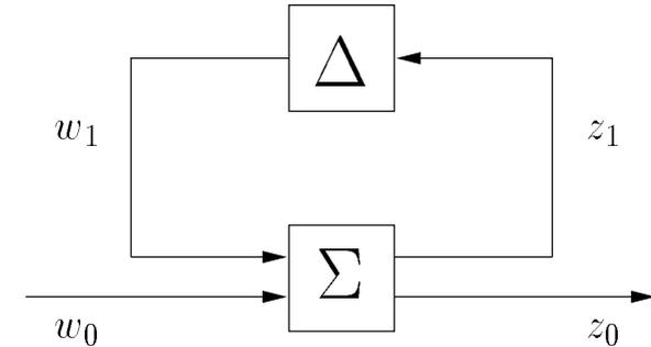
Figure 3.4: Setup for robust performance analysis.
