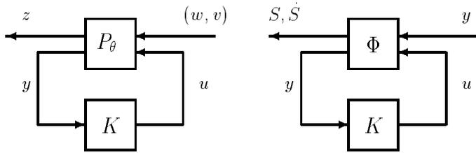
Figure 4.3: The original output feedback problem and the equivalent full information problem of controlling the total cost.
