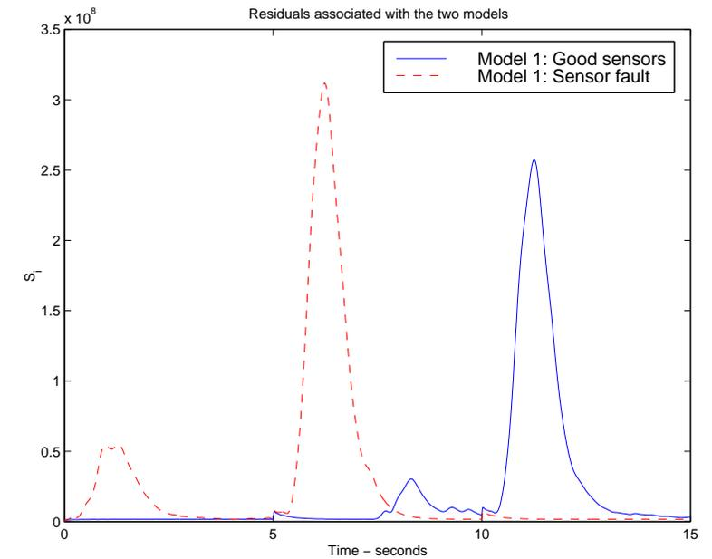
Figure 4.6: The residuals associated with the two models. The controller corresponding to the lower residual is connected to the plant. The fault at time 7.4 seconds is detected when the lines cross; approximately at time 7.6 seconds.
