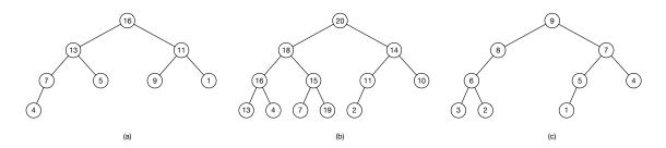
**1.2** [w] Which of the following arrays are heaps? Index 0 is not used and is therefore marked with —
